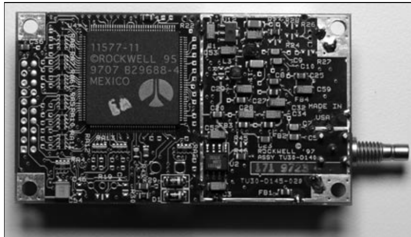
Figure 2. The Rockwell "Jupiter" GPS Receiver (-211) With Right Angle OSX (Bottom View -- Shown Approximately Twice Actual Size)
